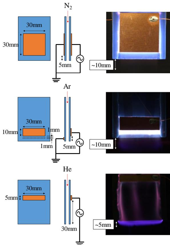
Fig.2. Structure and photographs of line type atmospheric pressure plasma jets
