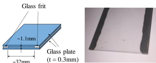
Fig.1. Structure and photograph of rectangular tube
