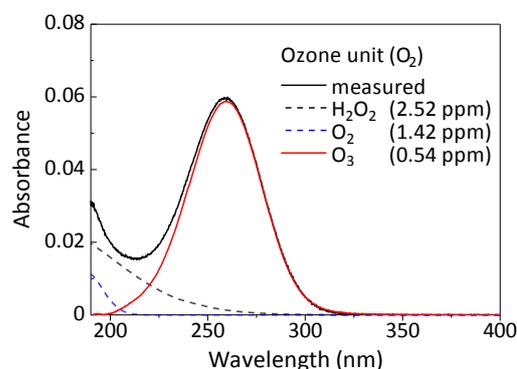
**Fig. 1** UV absorption spectrum of ozonated water with curve fitting results.
